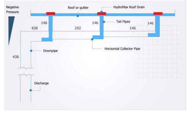
The pipe is installed flat without slope to quickly fill up with water. Once all of the pipework in the system is completely full of water <u>the main vertical stack creates negative pressure</u> which starts pulling the water off the roof level in every direction.
