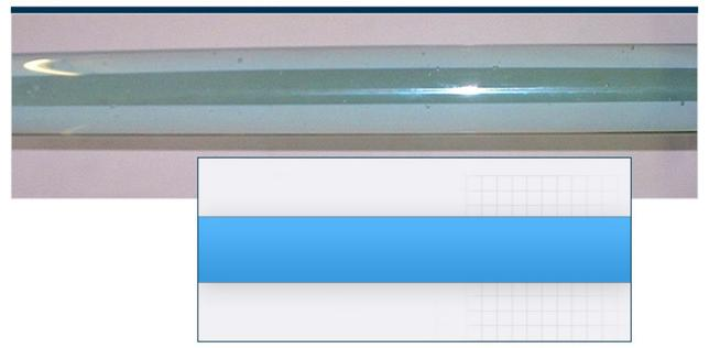
When the inflow is sufficient to maintain a water level above the roof drain air baffle, no air comes in and the system flows in full bore water flow; the pipework is 100% full of water.
