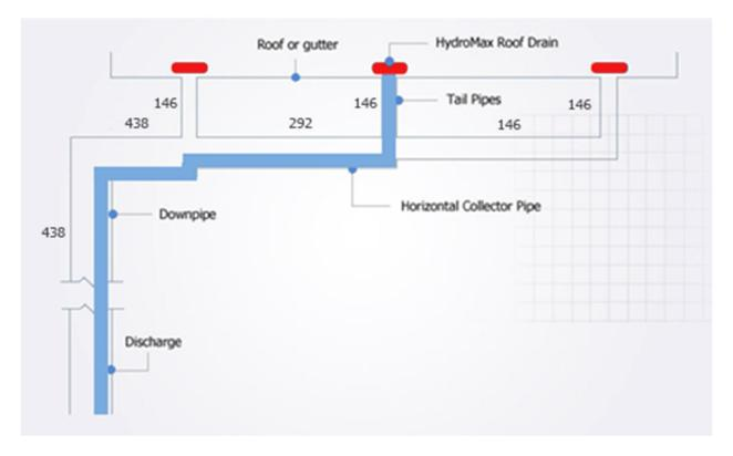
To prove this logic, we created a siphonic system on our MIFAB HydroTechnic Balancing Software using common tailpipe measurements the Engineer asked us to test: 24" initial vertical drop followed by 10' of horizontal pipe to discharge. For this calculation we are using a MH-301: 3" overflow siphonic drain sized to 146 GPM.
