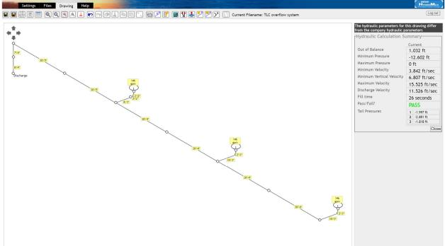
Again, we can see the green 'PASS', letting us know the system is 100% function, and fully compliant with the ASPE 45 Standard.
