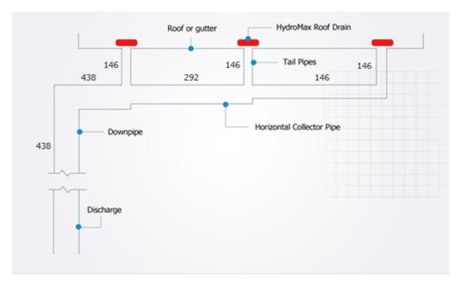
As the rain enters the HydroMax<sup>®</sup> roof drain, the tailpipes will quickly fill and supply water into the horizontal collector pipe. The tailpipe will continue to discharge water into the main horizontal collector pipe. As more water is supplied to the main horizontal collector pipe, the water will be in gravity flow with air and water mixing in the pipe as shown below.
