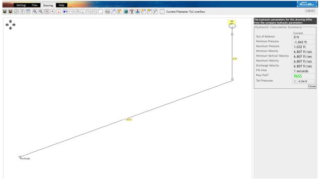
(Note: MH-301 can handle MAX 415 GPM which is just under 10,000 sq ft @ 4" rainfall rate.)
