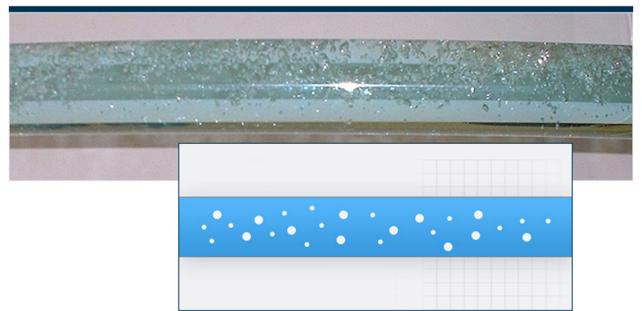
When more inflow comes and the roof drain prevents air ingress, the flow mostly fills the pipe but any air that does enter is transported in what is called bubble flow pattern.
