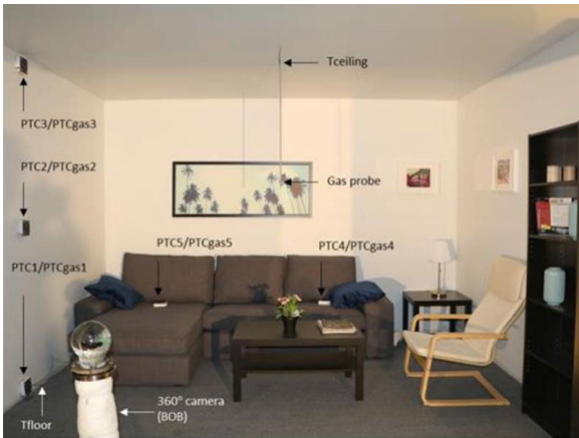
Figure F-4. Photo of NIST room fire test
