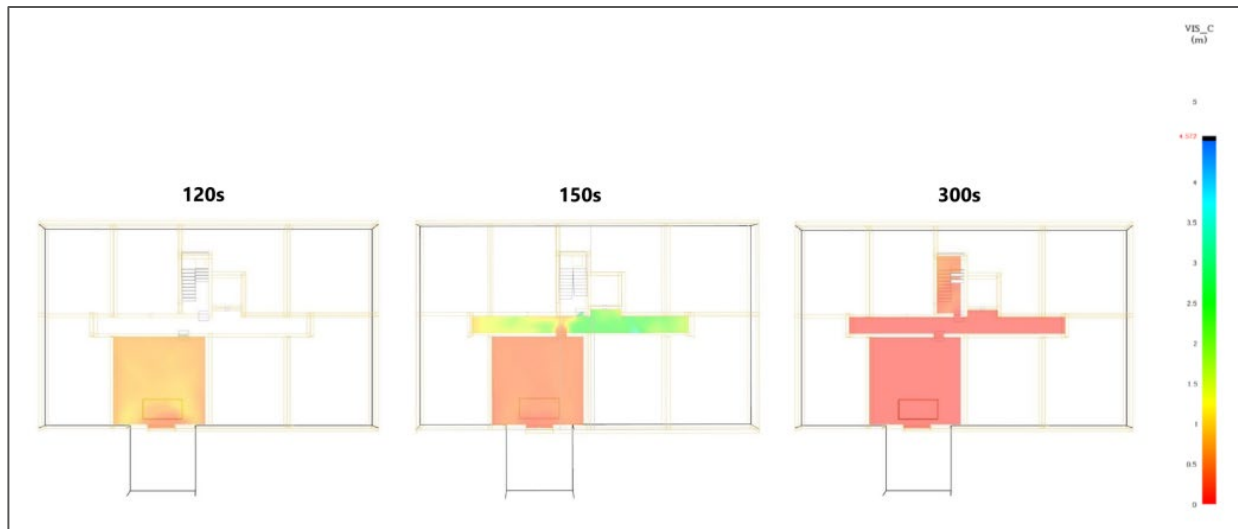
Figure H-21. Building 3, Scenario 3-2. Plan view of fire floor corridor visibility tenability criterion of 15 feet at 120 seconds, 150 seconds and 300 seconds
