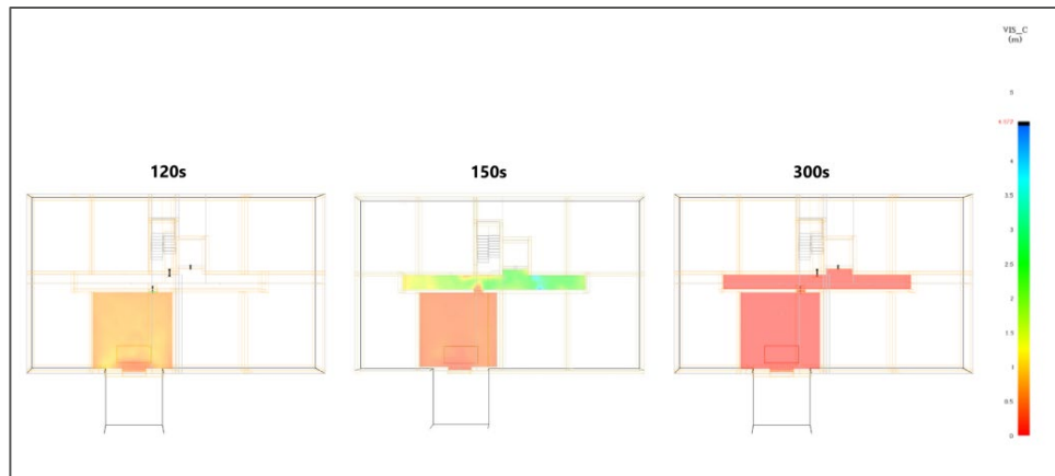
Figure H-19. Building 3, Scenario 3-1. Plan view of fire floor corridor visibility tenability criterion of 15 feet at 120 seconds, 150 seconds and 300 seconds
