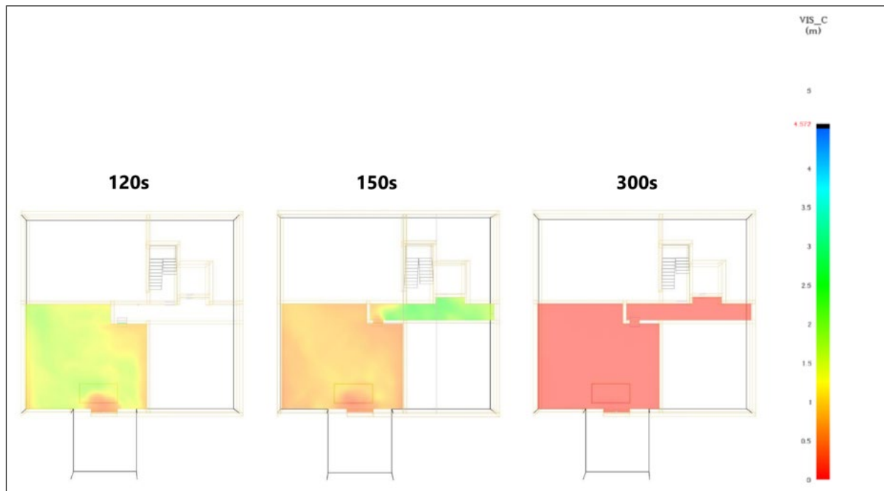
Figure H-11. Building 2 and 4, Scenario 2-1. Plan view of fire floor corridor of visibility tenability criterion of 15 feet at 120 seconds, 150 seconds and 300 seconds
