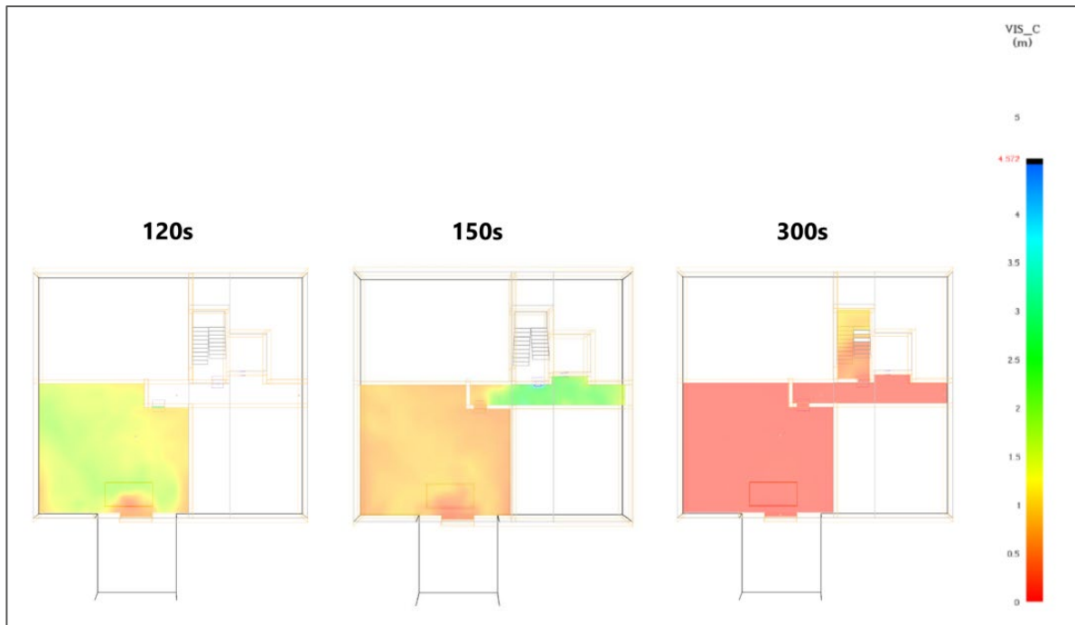
Figure H-15. Building 2 and 4, Scenario 2-2. Plan view of fire floor corridor visibility tenability criterion of 15 feet at 120 seconds, 150 seconds and 300 seconds
