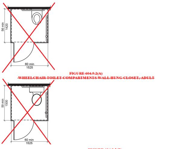
FIGURE 604.9.2(B) -WHEELCHAIR TOILET COMPARTMENTS FLOOR MOUNTED WATER CLOSET, ADULT - WALL HUNG AND FLOOR MOUNTED WATER CLOSET, CHILDREN
