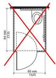
FIGURE 604.9.2.3 -WHEELCHAIR TOILET COMPARTMENTS ALTERNATE WHEELCHAIR TOILET COMPARTMENT
