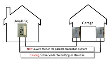
To ensure that neutral current is not continuously flowing on the new 4-wire feeder EGC, a new EGC would be required to be installed with the existing 3-wire feeder conductors, and installed according to NEC 300.3(B). The new EGC routed with the existing 3-wire feeder would be sized based on the overcurrent protection on the supply side of the feeder, according to NEC table 250.122. The equipment grounding conductors and neutral conductors would need to be separated
